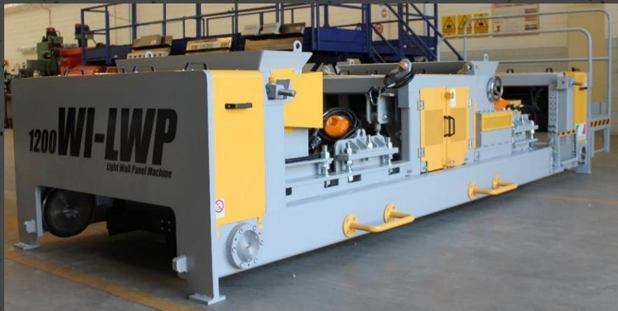
Witech LWP light wall clay panel machine, casting machine for manufacturing of non-load bearing, precast partition wall panels.
