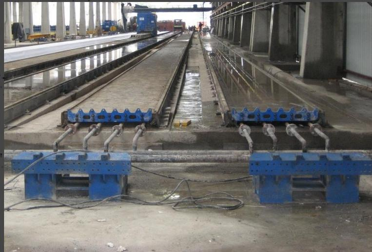
The bed is delivered in 12 m long sections, moulding surfaces are treated with the special agent for protection from the damages during transport.
