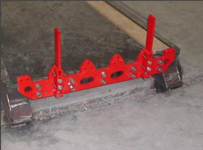
The strand spacer are used to keep the pre-stressing strands in the right position and are adjustable by height. They are build with strong steel and are mounted at the beginning of casting beds.
