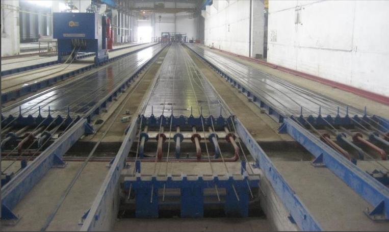
The casting bed consists of a construction of rolled steel profiles, with a surface plate of a special straight rolled and polished high-quality steel sheet, thick 8 mm.
