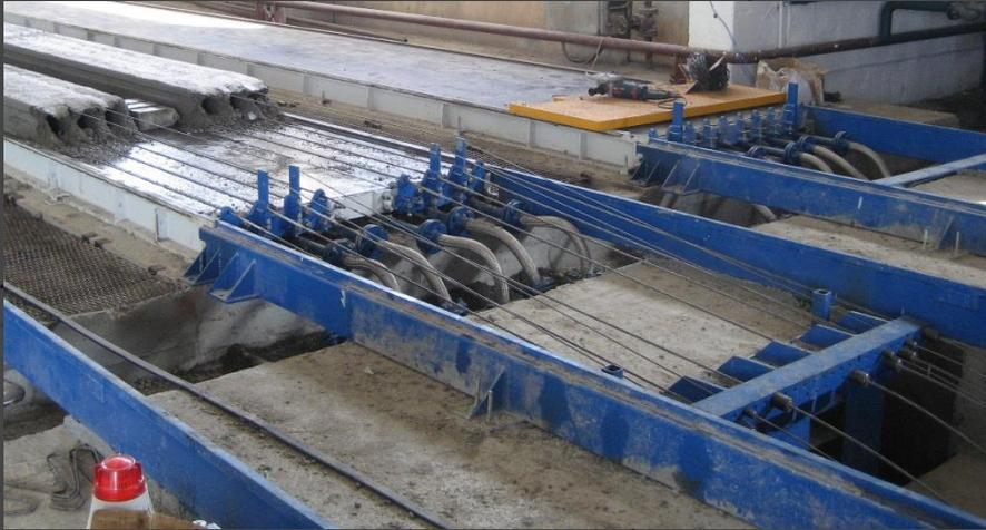
The exit bridges are needed to use the full length of the casting beds during the production. The exit bridges are special metal bridges for the correct exit of the machines at the end of the casting bed.
