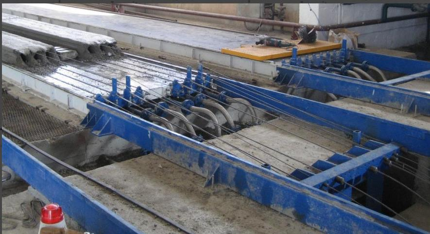
The exit bridges are needed to use the full length of the casting beds during the production.
