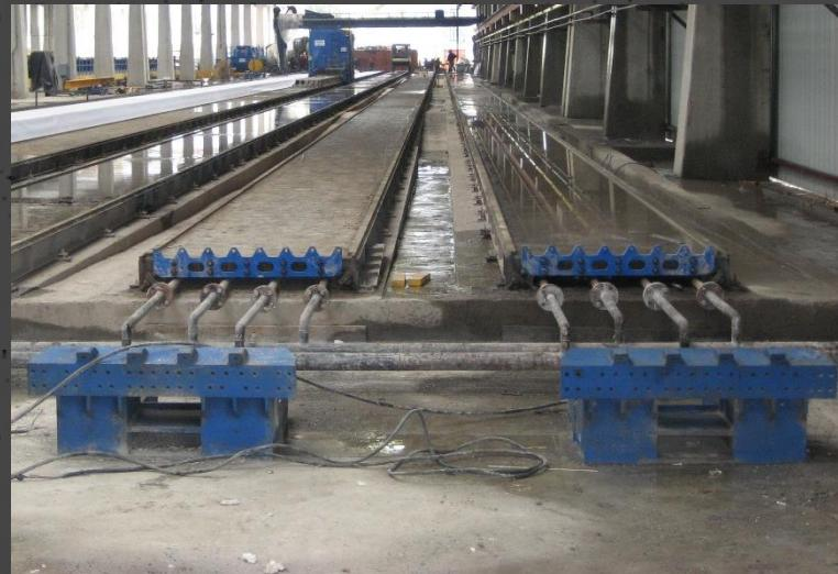
The casting bed consists of a construction of rolled steel profiles, with a surface plate of a special straight rolled and polished high-quality steel sheet, thick 8 mm.
