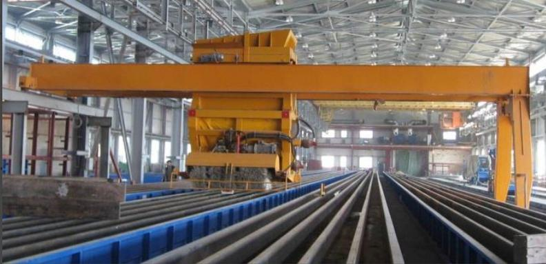
WiTech has specialized in the production of automatic and manual plants for the production of foundation POLES. It is equipped with an automatic system for distribution of the concrete in the formworks which are provided with heating system and automatic vibration.
