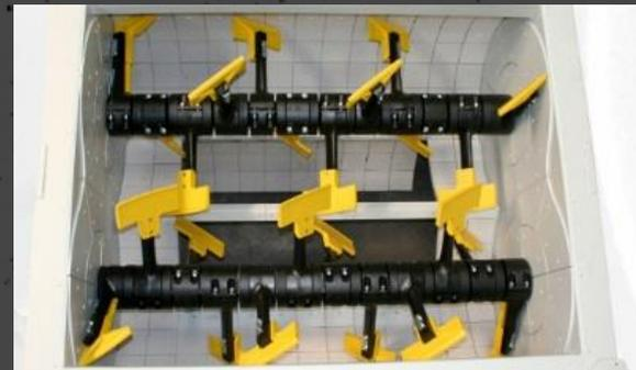
**Twin shaft mixers OW**, are specially made for the production of great amount of concrete and the main features are, high-speed mixing, quick discharge, low-cost production and quality of the mixing batch.
