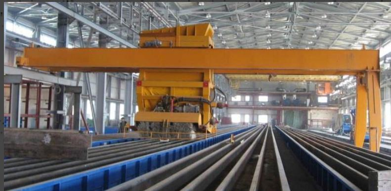
WiTech has specialized in the production of automatic and manual plants for the production of foundation POLES. It is equipped with an automatic system for distribution of the concrete in the formworks which are provided with heating system and automatic vibration.
