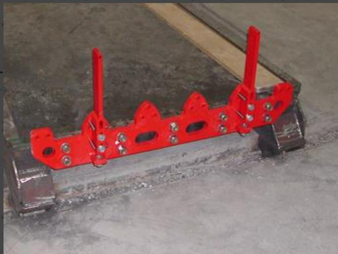
The strand spacer are used to keep the pre-stressing strands in the right position and are adjustable by height.
