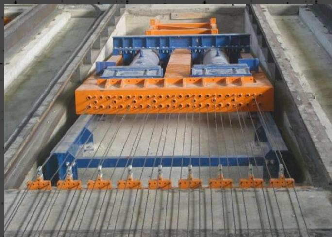
The timing for stressing the strand is around 2/3 minutes. This system is recommended when it is necessary to use many strands
